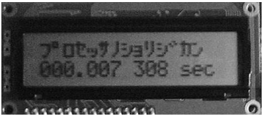
Fig. 13. LCD display (on board) for processing time
